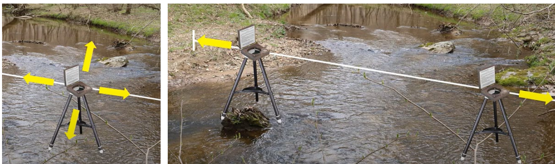
Densiometer set up for observations at mid-stream (A) and a single observation bankside (B). Photos: USWS.
