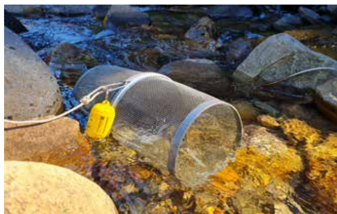
Minnow trap set in a stream. Placing rocks inside the trap will help weigh it down and the trap should be tied to a rock or wooden stake at the stream bank to ensure it remains secure.
