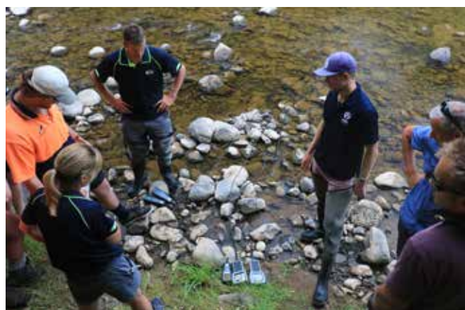
Environmental monitoring staff from NIWA and Otago Regional Council carrying out side-by-side field measurements (left) and water sample collection (right). The two samples were sent to the lab for nutrient testing to check there was close agreement in the results (as would be expected).
