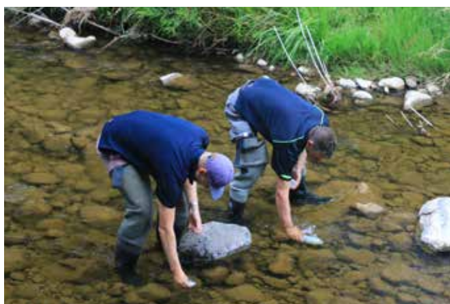
Environmental monitoring staff from NIWA and Otago Regional Council carrying out side-by-side field measurements (left) and water sample collection (right). The two samples were sent to the lab for nutrient testing to check there was close agreement in the results (as would be expected).
